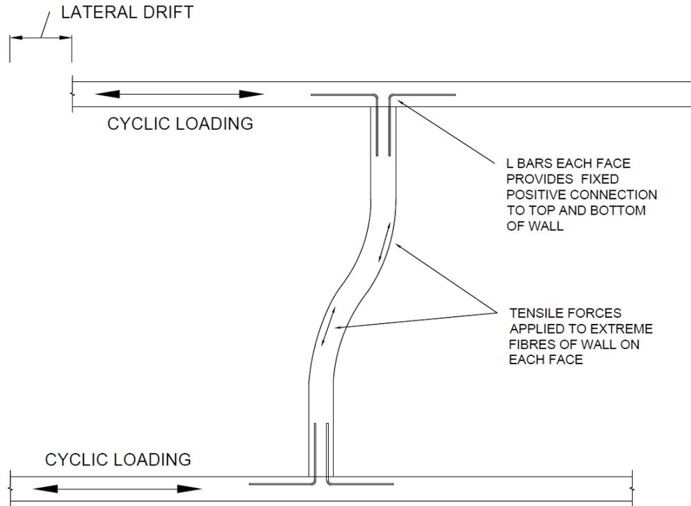
**Figure 2 – Idealised behaviour from walls with fixed connection to slabs ('L' bars to each face)**
