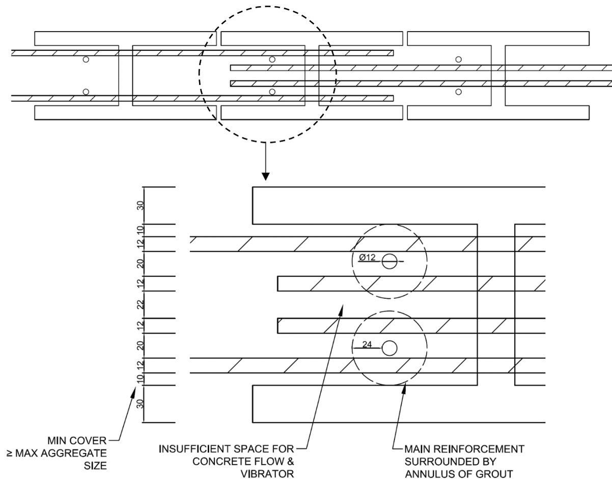
**Figure 3** – N12 Vertical and Horizontal Bars each face within a 20.48 'H' Block, at location where horizontal bars are spliced.
