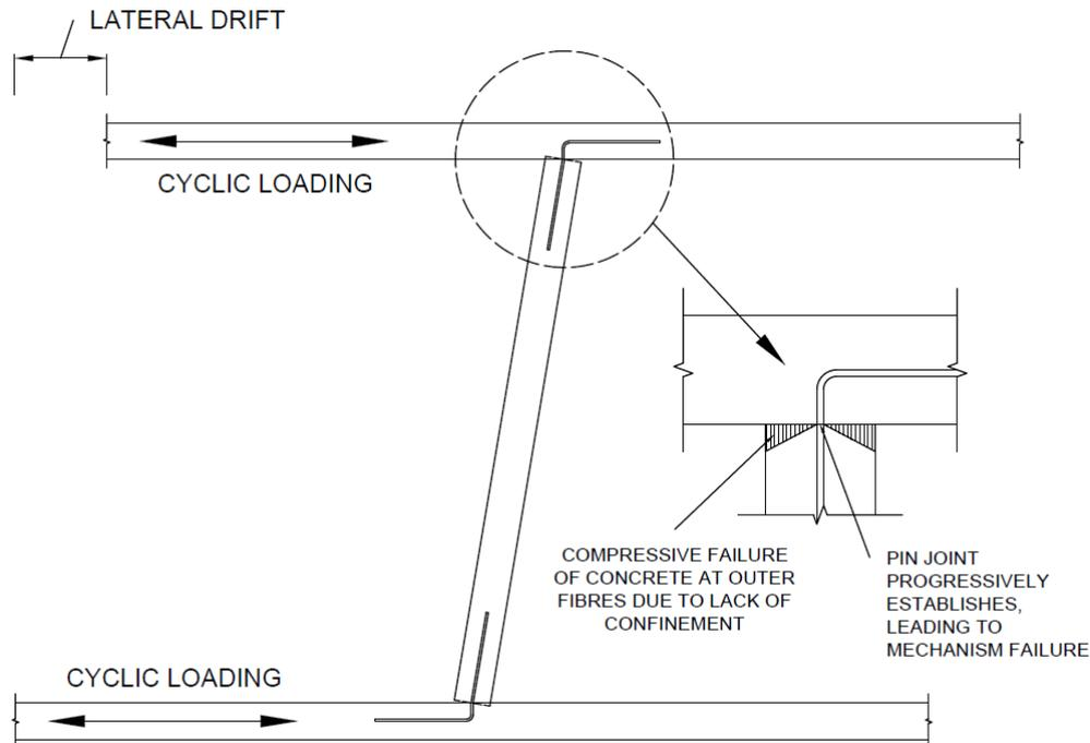
**Figure 1** – Idealised behaviour from walls with pin connection to slabs (central 'L' bars)
